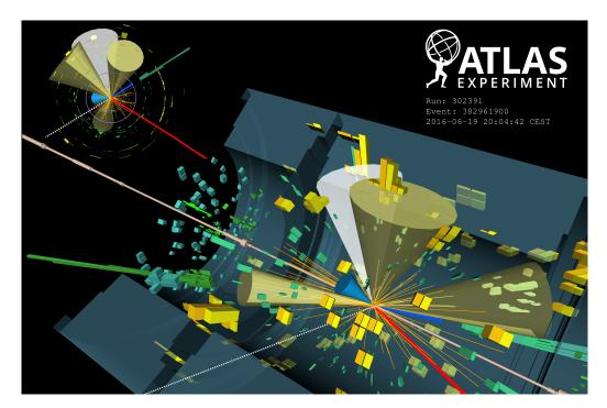
Figure 2: Event display of one of the candidate event in  $2\ell 1\tau_{had}$ . The blue track is the selected electron; the red track is the selected muon; the white cone is the  $\tau_{had}$  candidate; the three yellow cones are the selected jets and azure cone is the selected b-tagged jet. The green and yellow bars indicate the energy deposits in the electromagnetic and hadronic calorimeters [3].
