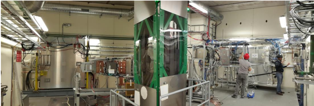
Figure 6 Inside view of the upstream irradiation field. Several detectors are visible. The ^{137}\text{Cs} irradiator is also visible in the foreground.
