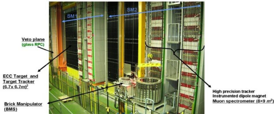
Figure 1. The OPERA detector.
