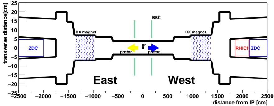
**Figure 2:** Location of the RHICf detector in the vicinity of the STAR experiment.
