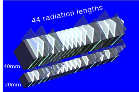
**Figure 1:** Schematic view of the RHICf detector composed of two compact sampling calorimeters.
