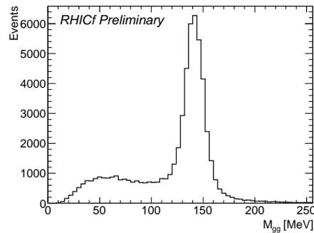
**Figure 7:** Distribution of invariant mass determined using photon pair events.
