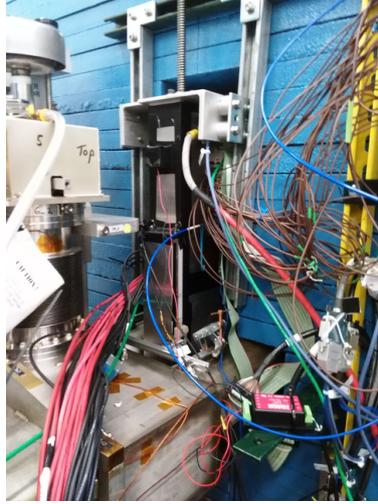
**Figure 3:** The RHICf detector installed in the RHIC tunnel.
