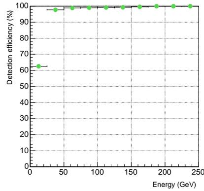
**Figure 4:** Detection efficiency in percent for photon incident as a function of photon energy in GeV.
