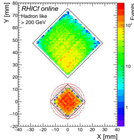
**Figure 6:** Hit map of high-energy neutrons when the small calorimeter was placed at the geometrical zero degree.
