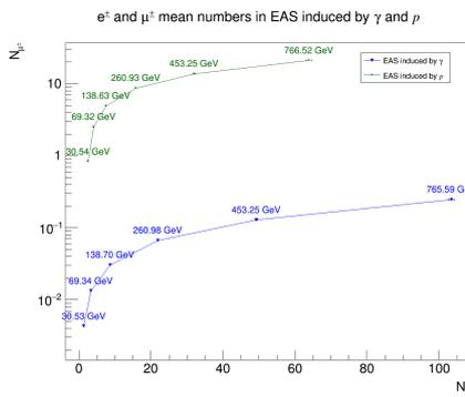
Figure 11: Mean value of  $e^\pm$  and  $\mu^\pm$  produced in EAS induced by primary  $p$  in function of primary particles energy.
