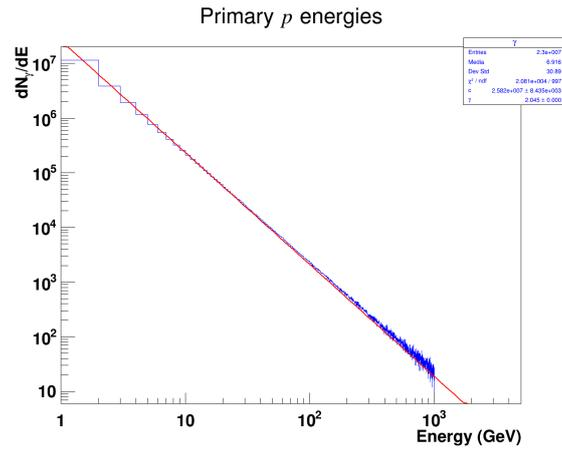
Figure 4: Protons simulated energy spectrum.
