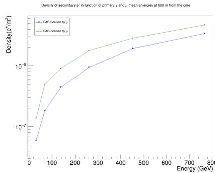
Figure 15: Secondary  $e^\pm$  density in function of primary  $\gamma$  and  $p$  energy at 600 m from the core.
